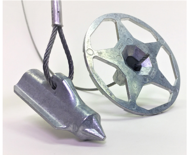
The tapered nose of the Falcon anchor head are designed to penetrate the soil with a sharp driving edge without deflecting, resulting in improved installation.
